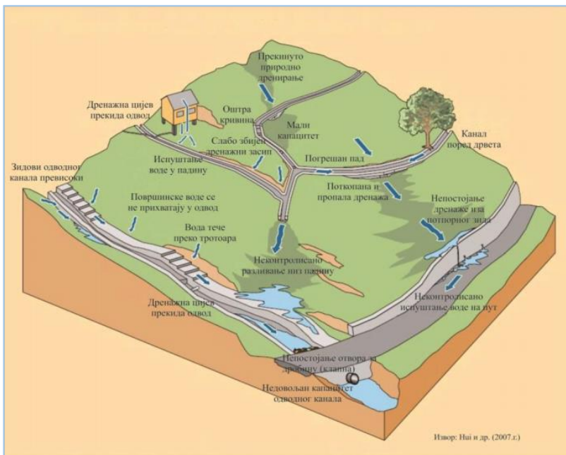
Figure 51: Poorly constructed drainage as a factor of instability 64
